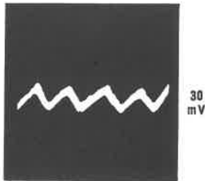
Fig. 4-8 210V Test Point
