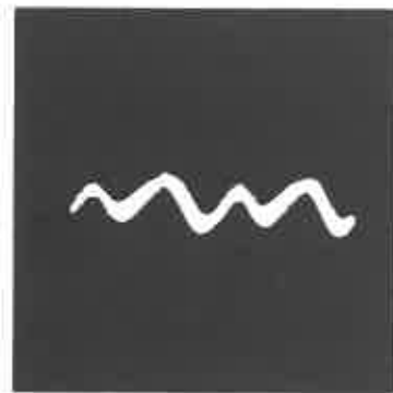
Fig. 4-10b Out of balance (approx. 450-500v peak to peak)
